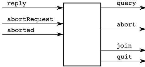
**Fig. 1.** Component interface (service part) for P2P algorithms
