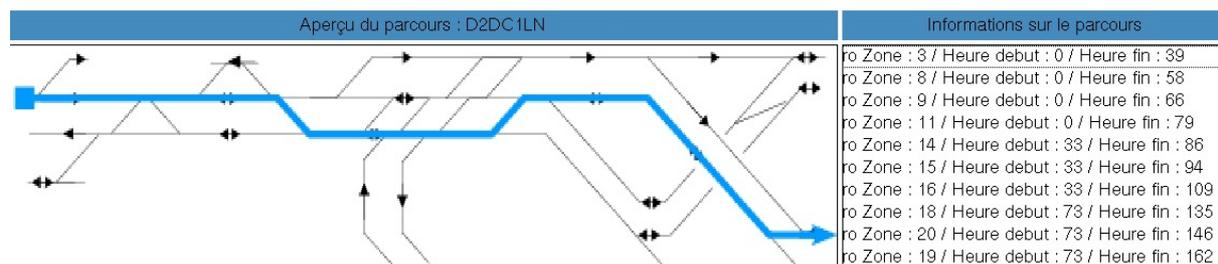
Figure 1: Visualization of a route through the infrastructure (left) and its associated description in terms of track sections occupation (right, in French)
