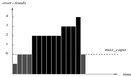
**Fig. 1.** The solution with values  $(0, 0, 0, 0, 2, 2, 2, 2, 2, 2, 3, 3, 3, 4, 0)$  w.r.t. cost variables  $X$  (the over-loads) strongly violates rules 2 and 3 although it satisfies the constraint  $Gcc(X, T, I)$  with  $T = (0, 1, 2, 3, 4)$  and  $I = ([5, 15], [0, 10], [0, 6], [0, 3], [0, 1])$ .
